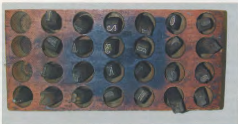
Parts of a ship had to be indented and this letter stamp kit was just the thing for it. A complete set would include all letters of the alphabet and zero through nine in numbers. Each letter would then be hammered in. (Photo by Mike Taylor)
