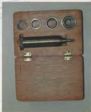
This is a center hole punch tool. Made of brass and steel, this tool allows a constructor to form perfectly centered smaller holes inside bored out larger holes. (Photo by Mike Taylor)
