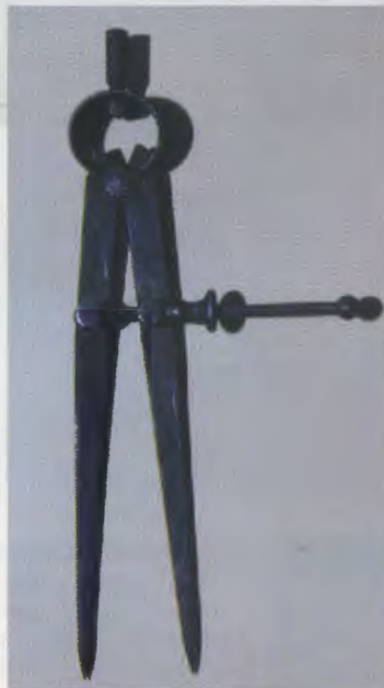
This is Hart's pair of dividers which would be used in layout work. They could have been used in both steel and wood work projects. (Photo by Mike Taylor)
